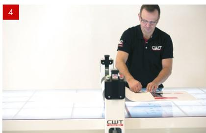
4 Pull the adhesive material halfway over the roller.
