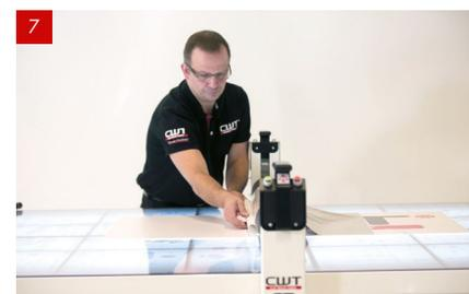
7 Fold the liner under the roller.
